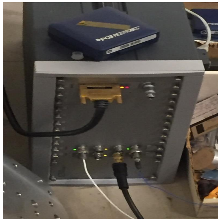
Figure 17, CPU of the control PC connecting the accelerometer with the PCB
