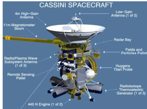
Figure 2.4.4. The Cassini/Huygens spacecraft and its principal features.
